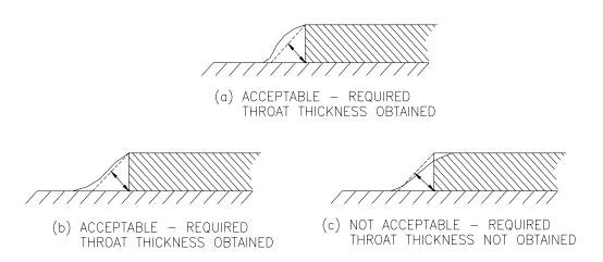
FILLET WELD EQUAL TO THE SIZE OF PLATE OR SECTION FIG. -16
