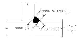
DIAGRAM OF WELD PASS IN FILLET WELD SHOWING DEPTH OF FUSION WIDTH IN CROSS SECTION  ${\rm AND} \ \ {\rm WIDTH} \ \ {\rm OF} \ \ {\rm FACE}$
