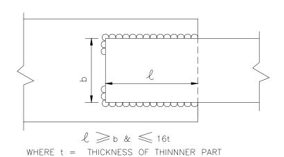
FILLET WELDS IN LAP JOINTS
