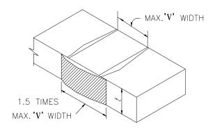
BUTT WELD END REINFORCEMENT FIG. -9
