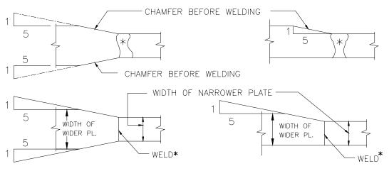
TRANSITION BY CHAMFERING THICKER OR WIDER PART  ${
